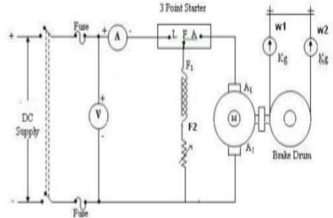
**Precaution:** While performing this test with series machines care should be taken that brake applied is tight failing which the motor will attain dangerously high speed and get damaged
