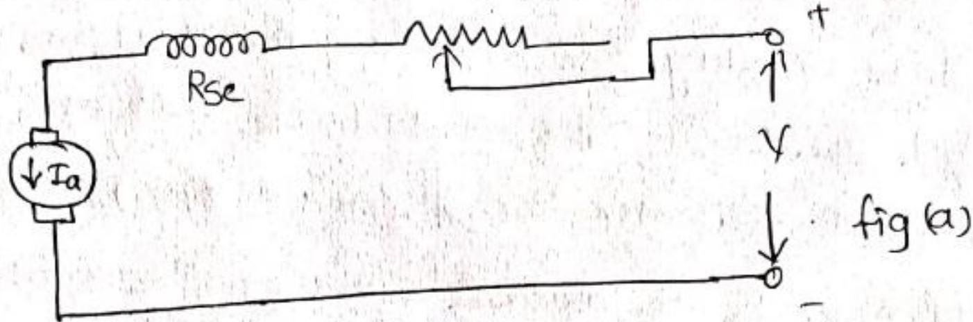
In this method, a variable resistance is directly connected in series with the supply to the complete motor as shown in fig(a). This reduces the voltage available across the armature and hence the speed falls. By changing the value of variable resistance, any speed below the normal speed can be obtained. This is the most common method employed to control the speed of the DC Series motor.
