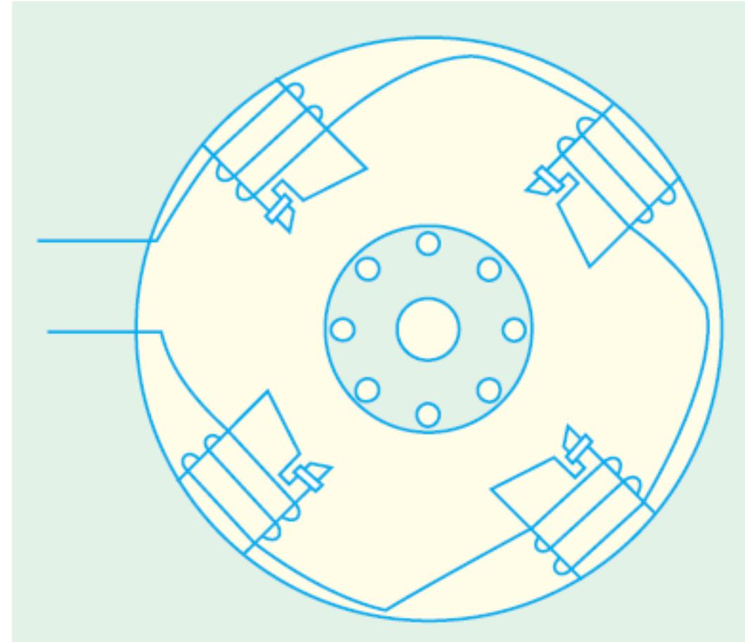
Rotor – The shaded pole motor uses the squirrel cage rotor.
