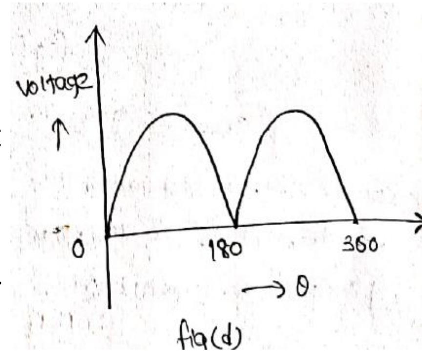
This is not a steady direct voltage but has a pulsating character. It is because the voltage appearing across the brushes varies from zero to maximum value and back to zero twice for each revolution of the loop.
