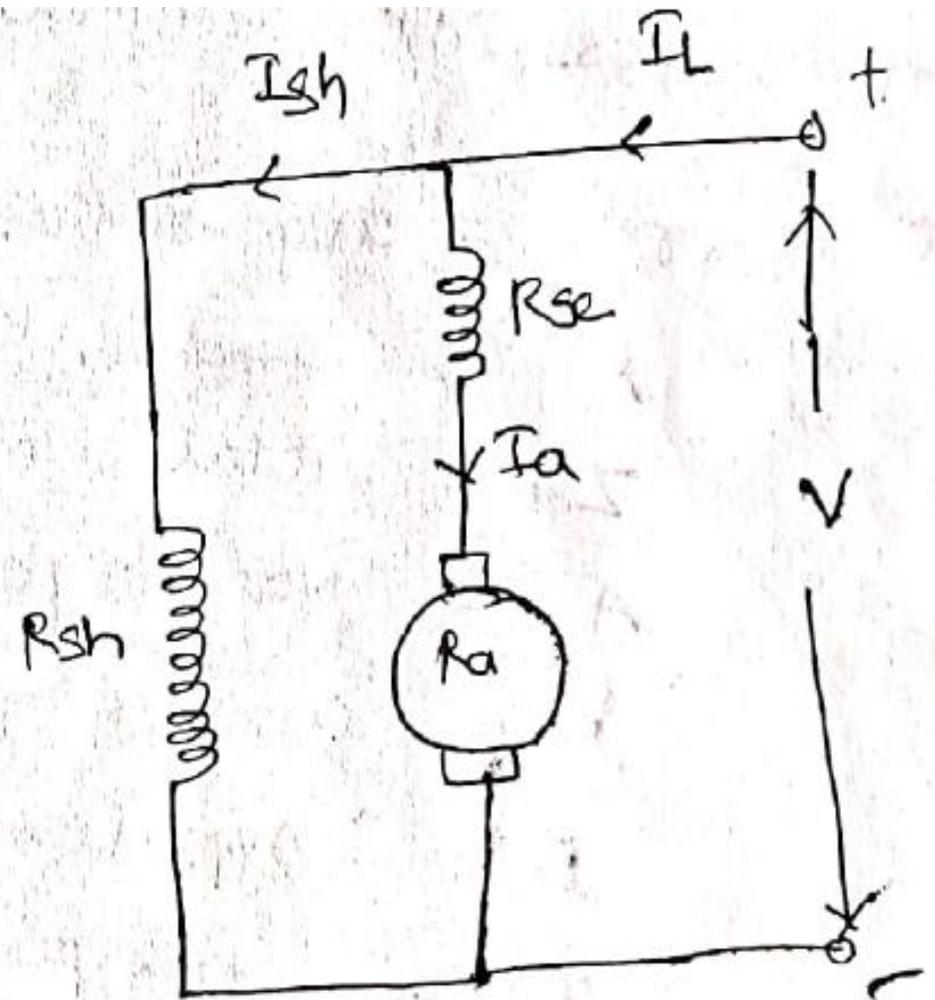
Fig(b) Long shunt motor
