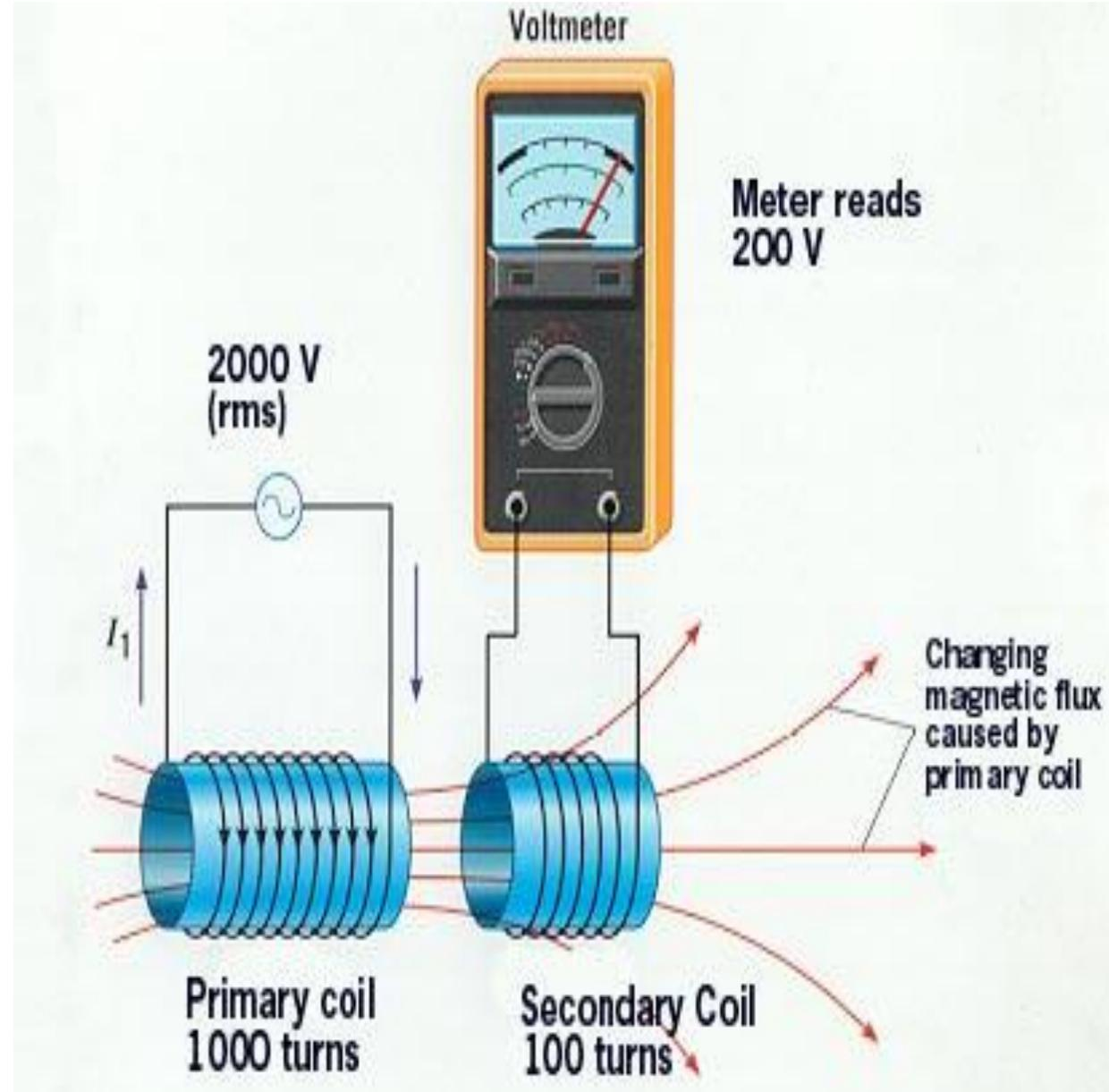
Because of this induced e.m.f., a current  $I_2$  will flow through the load connected with the secondary winding. The load terminal voltage is  $V_2$ .
