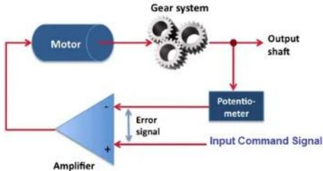
As the position of the potentiometer knob changes there will be an electrical signal produced at the potentiometer port. As the angular position of the potentiometer knob progresses the output or feedback signal increases. After desired angular position of motor shaft the potentiometer knob is reaches at such position the electrical signal generated in the potentiometer becomes same as of external electrical signal given to amplifier.
