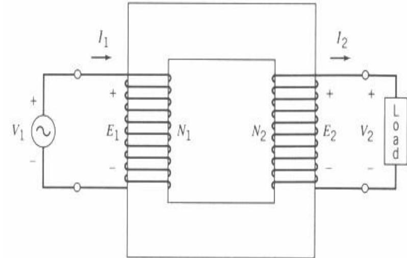
FIGURE 4.8 A transformer circuit.
