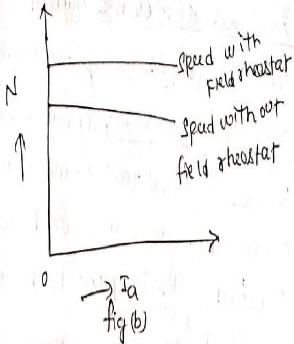
By varying the flux  $\phi$ , the motor speed ( $N \propto \frac{1}{\phi}$ ) can be changed and hence the name flux control method. In this method, a variable resistance (known as shunt field rheostat) is placed in series with shunt field winding shown in fig (a).
