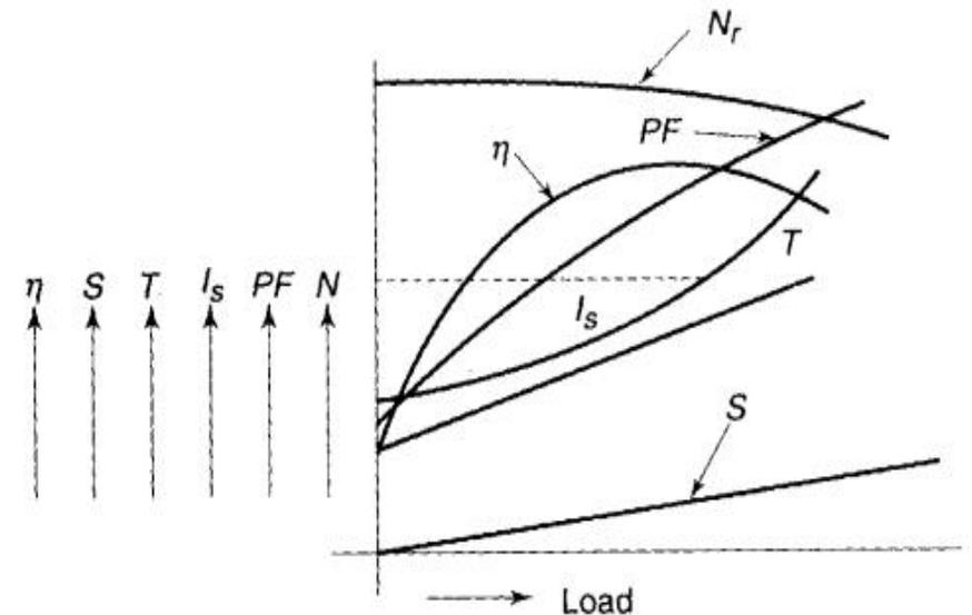
Graphical representation of the effect of load on rotor speed, efficiency power factor, output torque, stator current and slip of an induction motor.
