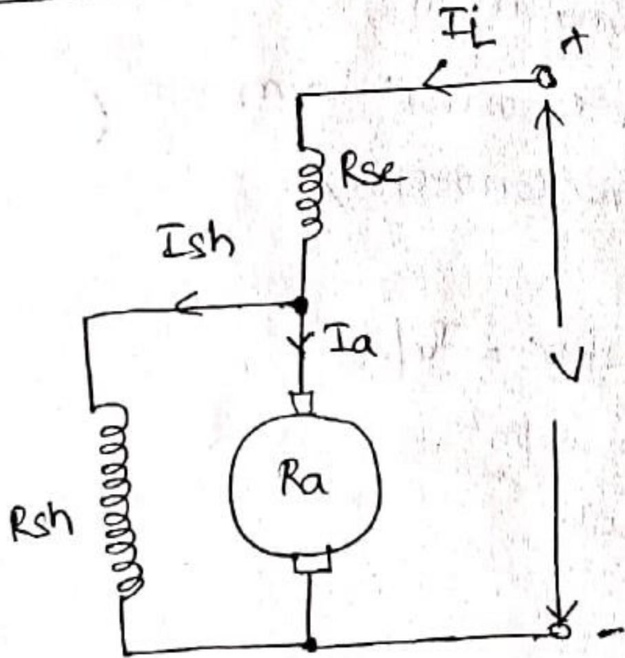
Fig(a) Short shunt motor
