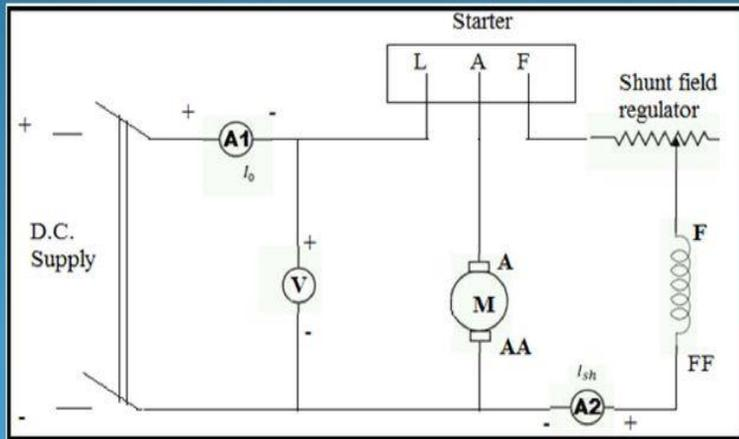
fig (A) circuit diagram of Swinburne's test on dc shunt motor
