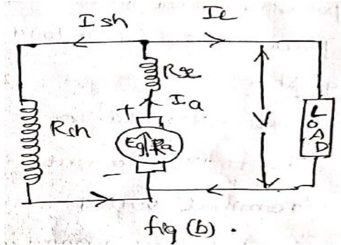
In a compound wound generator, there are two sets of field windings on each pole-one is in series and the other in parallel with the armature. A compound generator may be:
