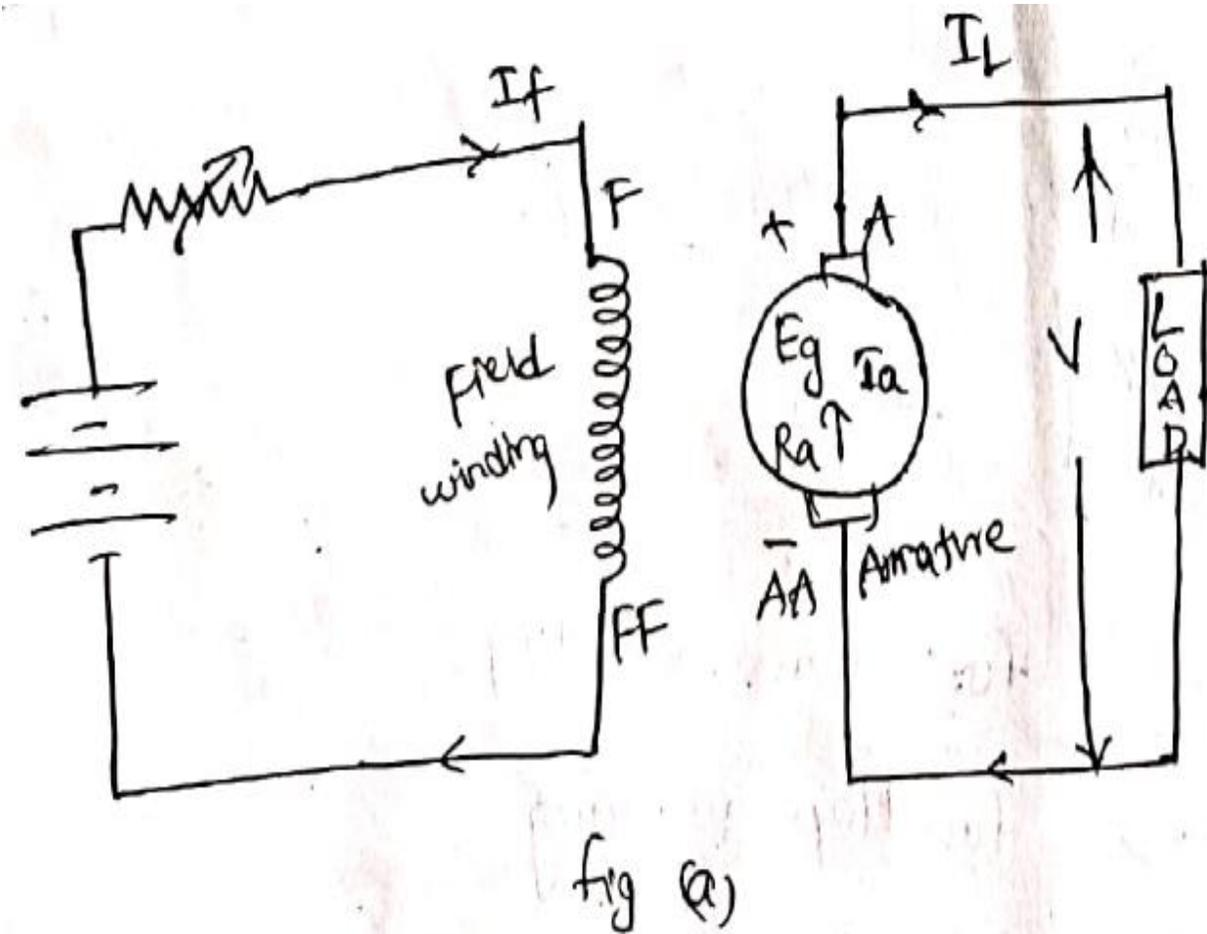
$$\begin{aligned}\text{Armature current} &= I_a = I_L \\ \text{Terminal voltage} &= V = E_g - I_a R_a \\ \text{Electrical power developed} &= E_g I_a \\ \text{power delivered to load} &= E_g I_a - I_a^2 R_a = I_a (E_g - I_a R_a) = V I_a\end{aligned}$$
