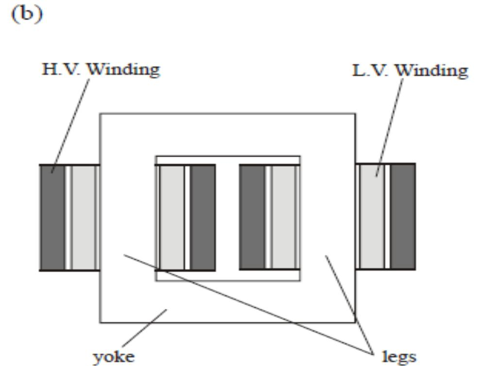
(a) Shell-type transformer, (b) core-type transformer
