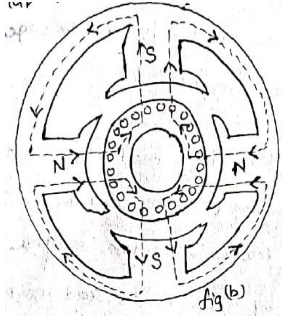
**Rotor is rotating part - armature**
