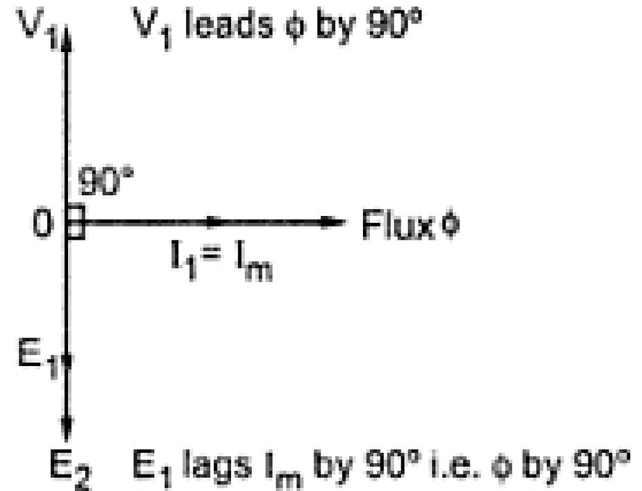
$V_1$  - supply voltage;
