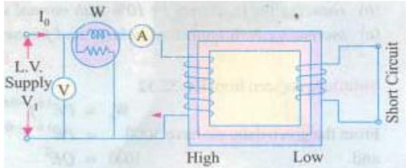
$$\text{Full load cu loss} = W_{sc} = I_{sc}^2 R_{01}$$
