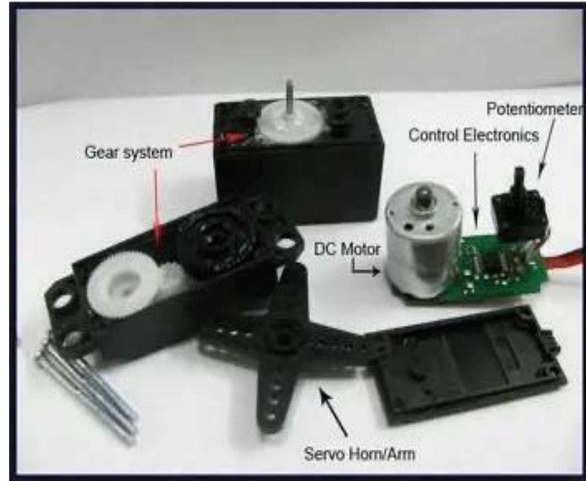
This is where the gear system inside a servomechanism comes into the picture. The gear mechanism will take high input speed of the motor (fast) and at the output, we will get an output speed which is slower than original input speed but more practical and widely applicable.
