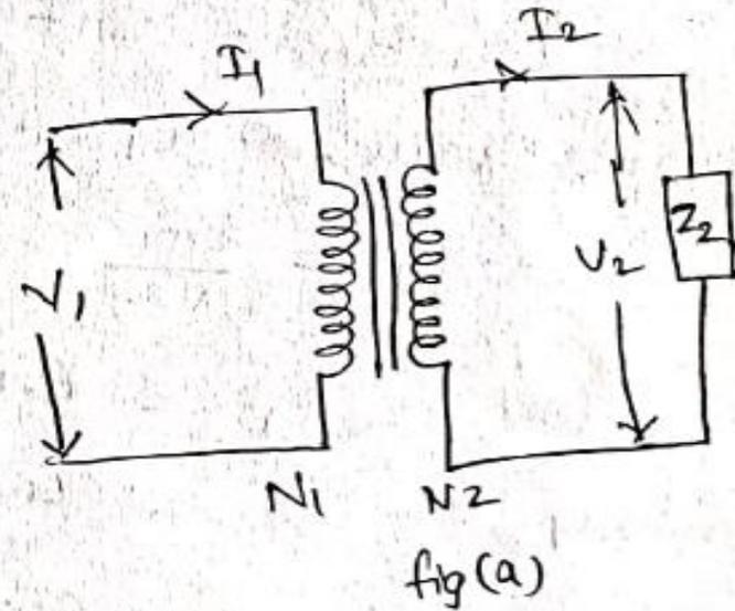
$$\left[ \because \frac{V_2}{V_1} = \frac{I_1}{I_2} = K \right]$$
