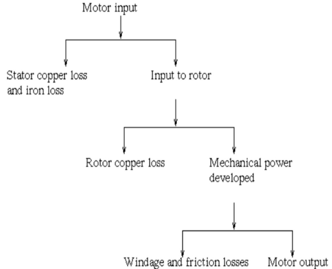
Electrical power input to the stator,  $P_{in} = \sqrt{3}V_L I_L \cos\phi$
