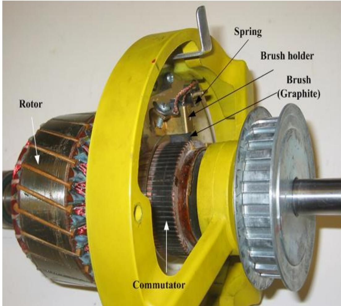
Cutaway view of DC motor
