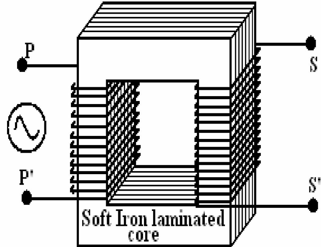
working :- when an alternating voltage  $V_1$  is applied to the primary, an alternating flux  $\phi$  is set up in the core. The alternating flux links both the windings and induces emf  $E_1$  and  $E_2$  in them according to Faraday's law of electromagnetic induction. The emf  $E_1$  is termed as primary emf and emf  $E_2$  is termed as Secondary emf.
