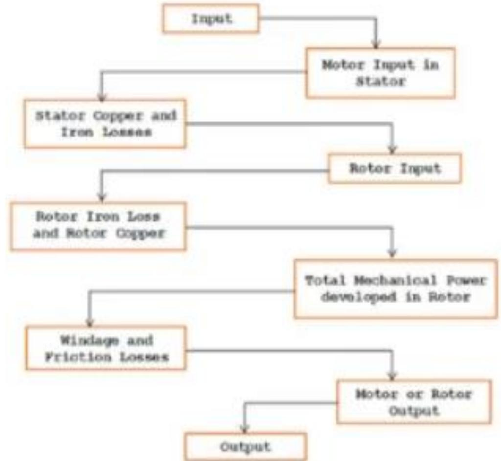
There are two types of losses occur in three phase induction motor. These losses are,
