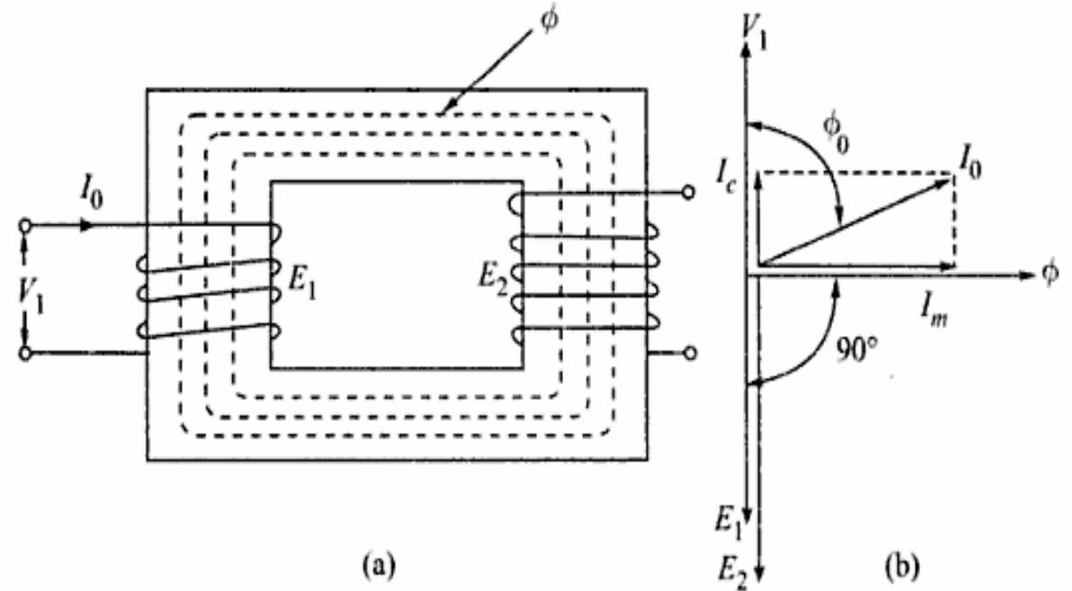
(a) Transformer on no-load (b) Phasor diagram of a transformer on no-load
