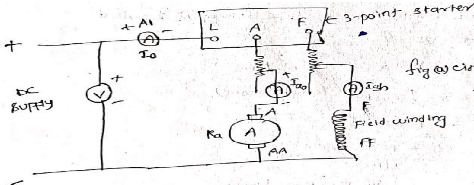
fig (a) circuit diagram for Swinburne's Test
