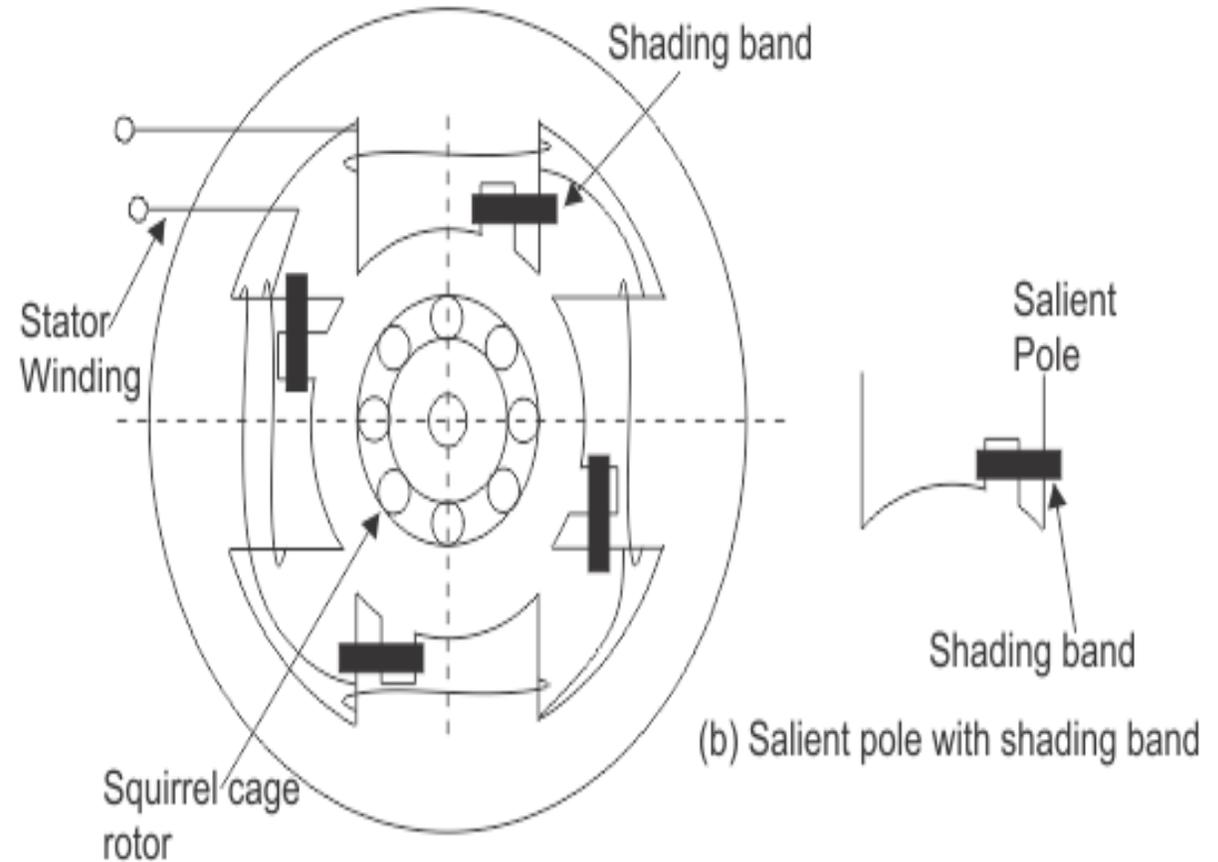
(a) 4-pole shaded pole construction
