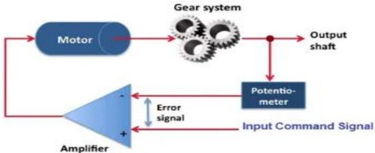
A servo system primarily consists of three basic components – a controlled device, a output sensor, a feedback system.
