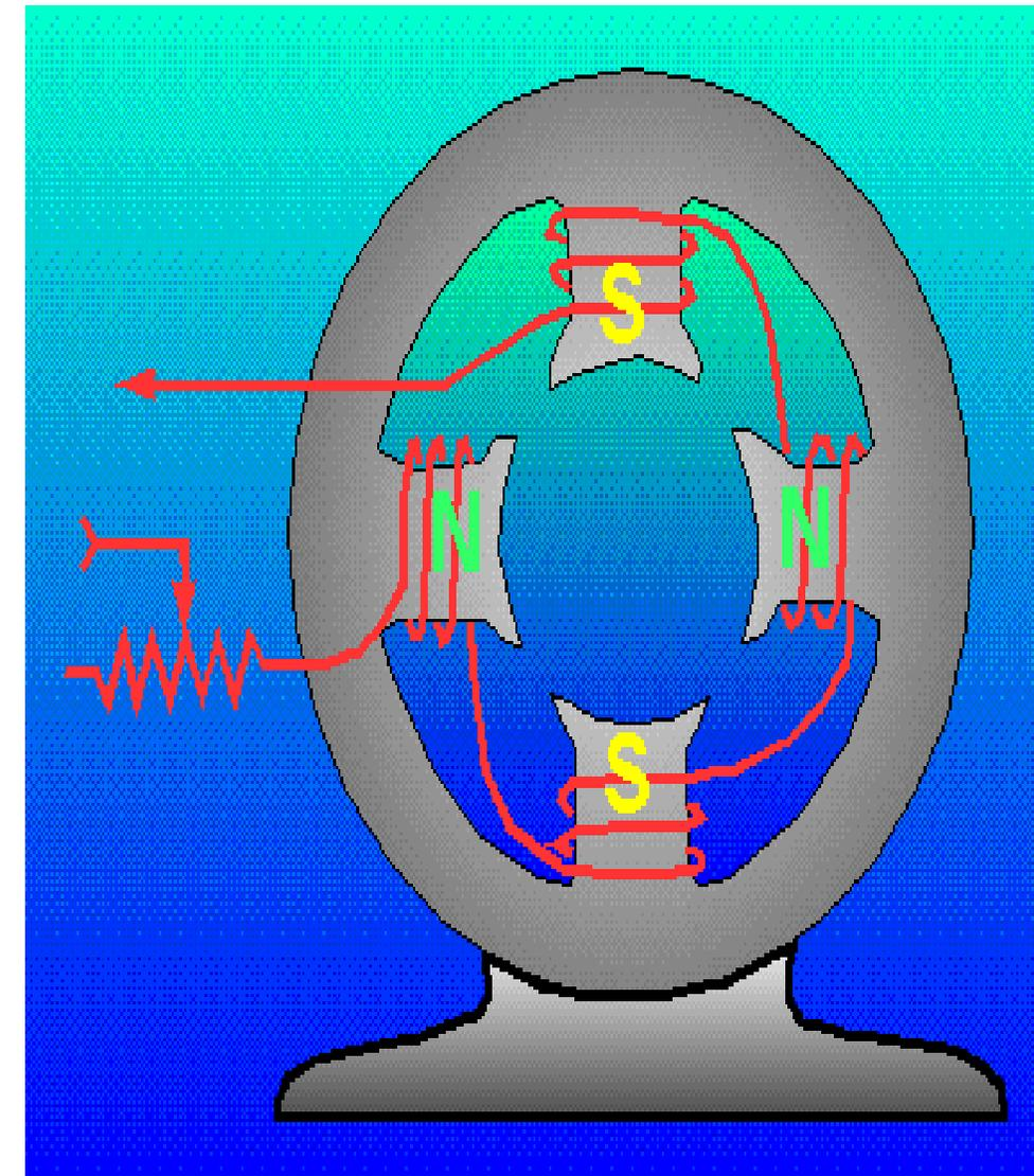
Four-pole generator(without armature)
