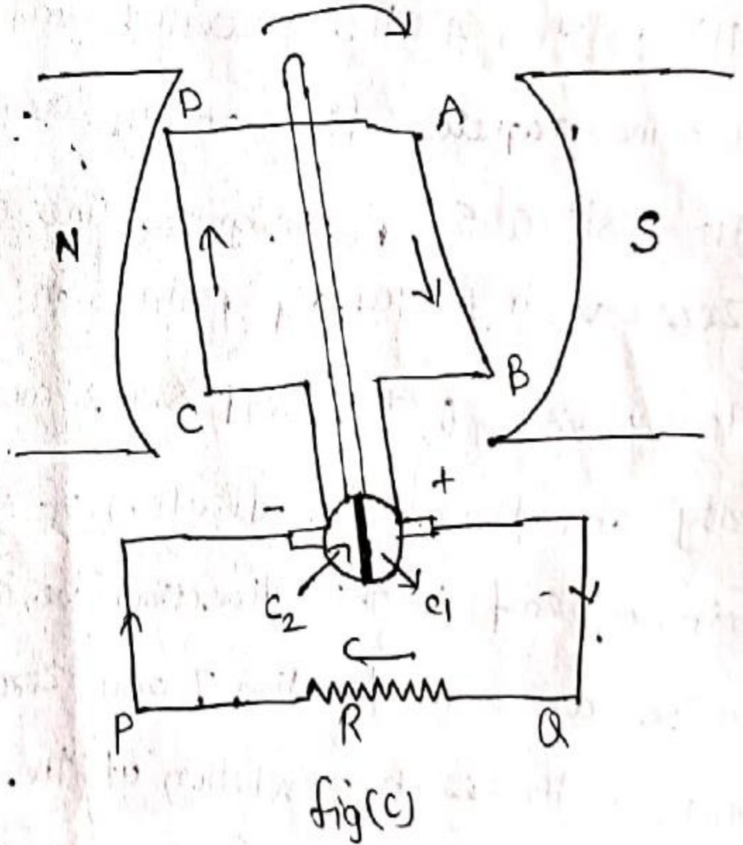
The commutator is mounted on, but insulated from the rotor shaft. **The ends of coil sides AB & CD are connected to the segments  $C_1$  &  $C_2$  respectively** as shown in fig(b). Two stationary carbon brushes rest on the commutator and lead current to the external load. **With this arrangement, the commutator at all times connects the coil side under S-pole to the +ve brush and that under N-pole to the -ve brush.**
