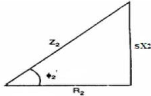
Induced emf per phase in rotor winding =  $sE_2$
