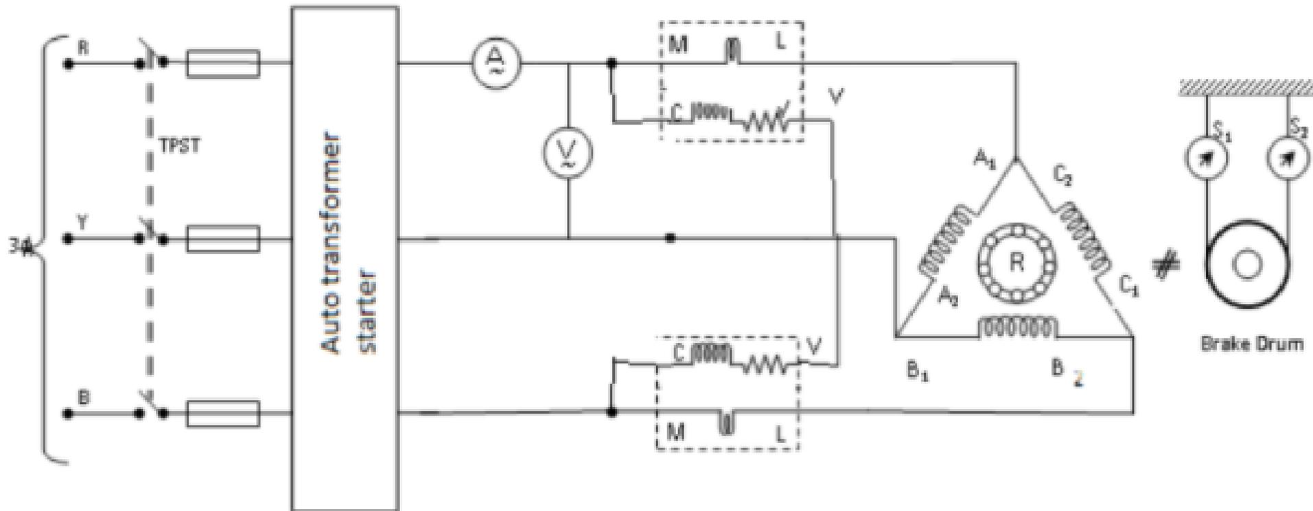
The load test on 3-phase induction motor is performed to obtain its various characteristics including efficiency. A belt and brake drum arrangement as shown in the circuit diagram can load the motor.
