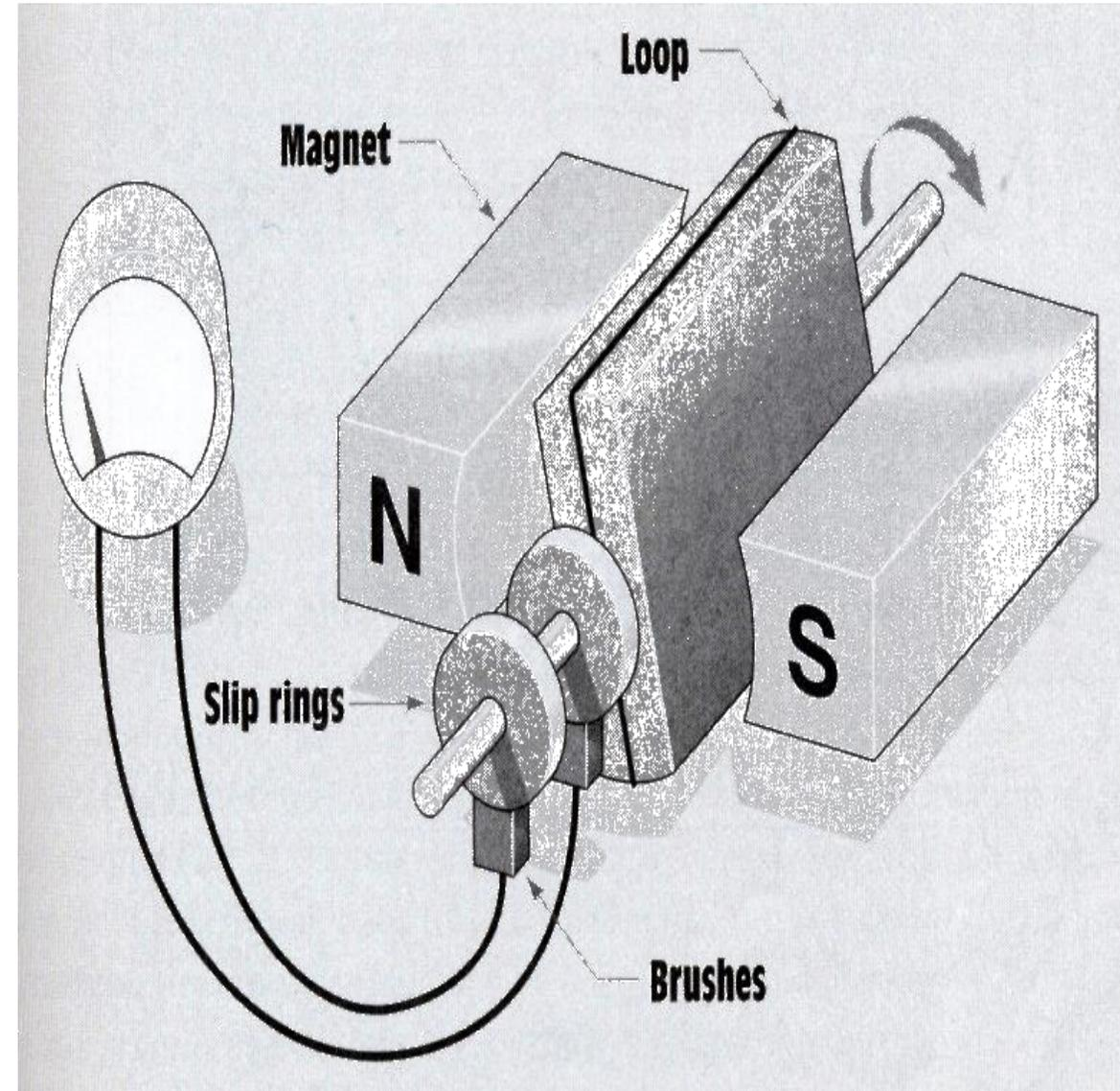
**Principle of magnetic induction in DC machine**
