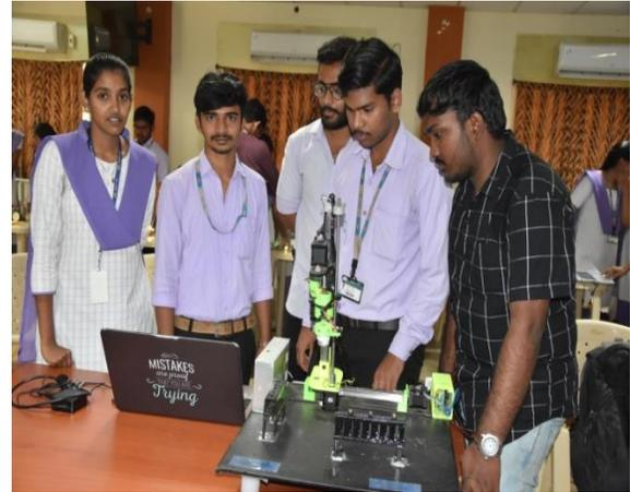
Prototype of Scara Robot
