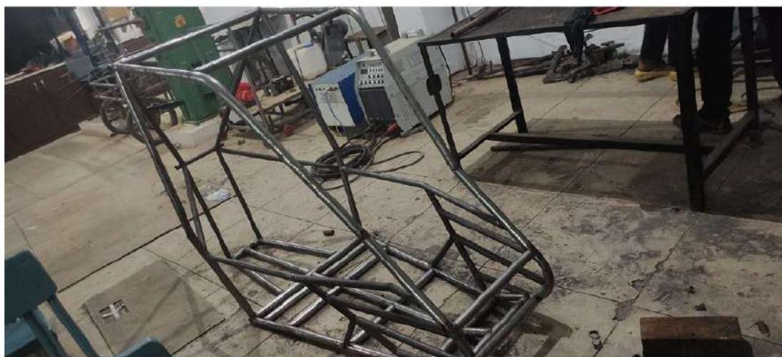
Figure 1 Fabrication of the ATV chassis
